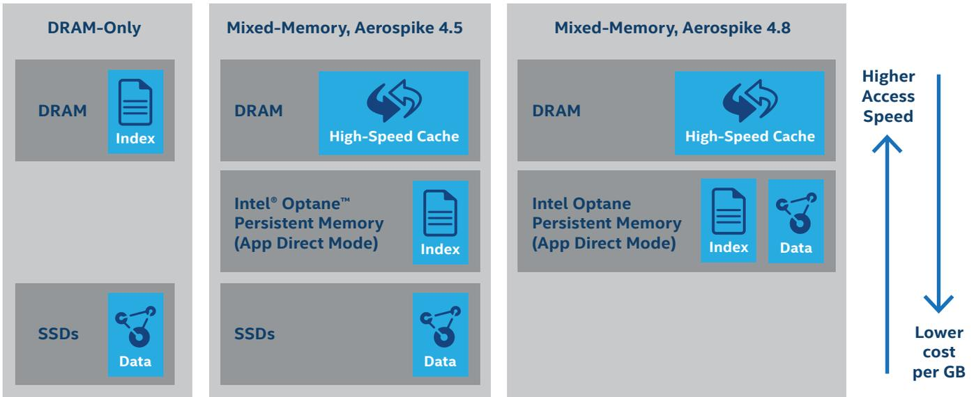
Figure 4. Evolution of Aerospike and Intel collaboration.
