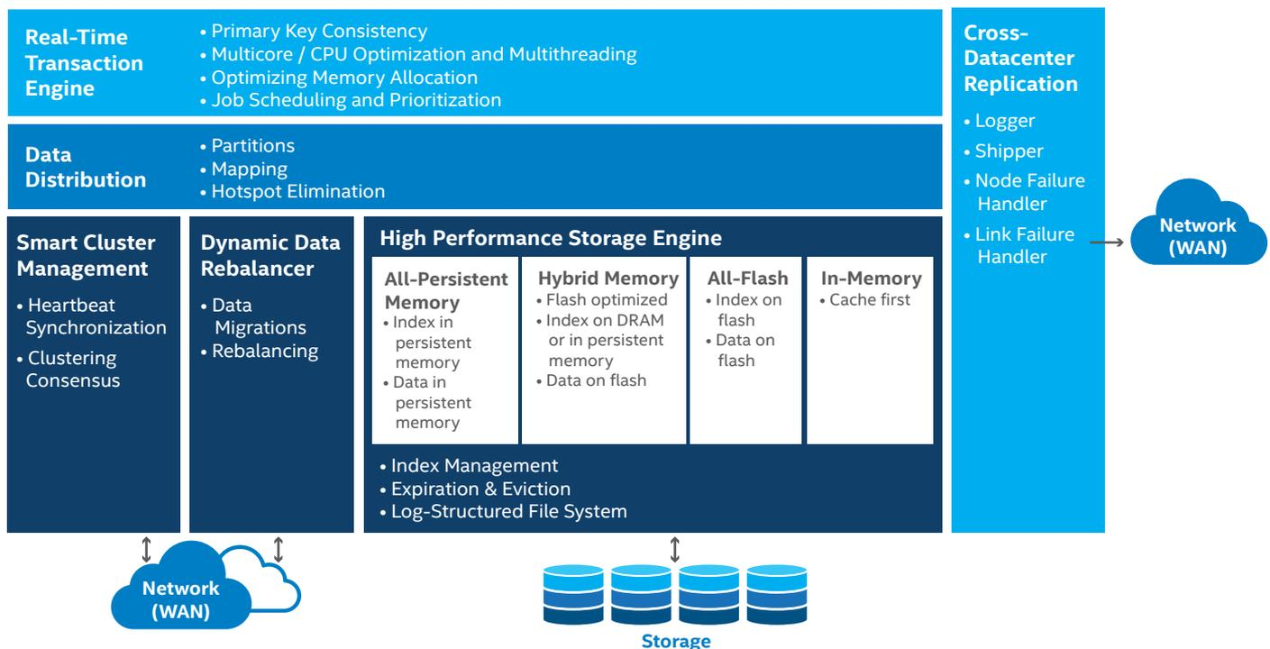
**Figure 1.** Aerospike 4.8 with Intel Optane persistent memory supports high volume, real time, mission-critical transactions and analytics operating on petabyte-scale data sets with mission-critical reliability.
